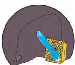
internal supply of coolant for machining austenitic stainless steel
