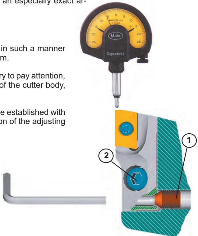
Such installation of mill is necessary only in case of high requirements to the surface by finishing with little allowances for machining. In all other cases remain the basic installation of cartridges with support on the face surface of cutter body produced by manufacturer.
