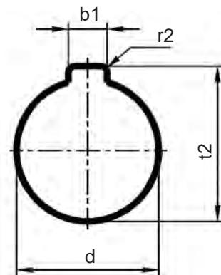
**Disk mills with drive slot to (type "F") DIN 138**
