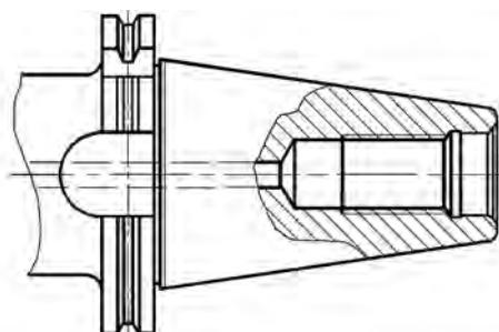
**NC...B** - 7/24 taper shank with coolant supply over shoulder DIN 69871 B
