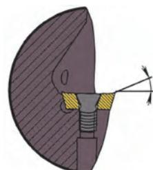
internal supply of coolant for machining of titanium alloys and high-temperature materials
