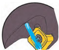
Internal coolant supply for machining austenitic stainless steel
