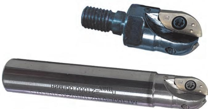
For correct assembly, the marks on the cutter body should match those on the insert
