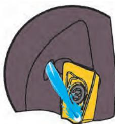
internal supply of coolant for machining austenitic stainless steel, titanium alloy
